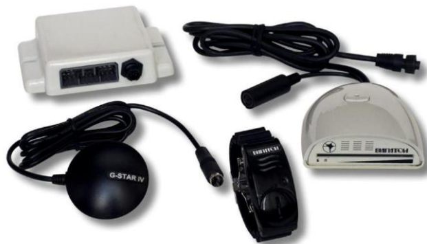
Fig 1. VIGITON system of driver's vigilance monitoring
